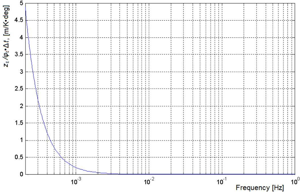
Fig. 1. An example of constructing of the noise transfer function generated by the crossed leaf rotary flexure, in relation to the amplitude of ambient temperature changes and the initial bending angle (for the seismometer SK-1 [1]).
