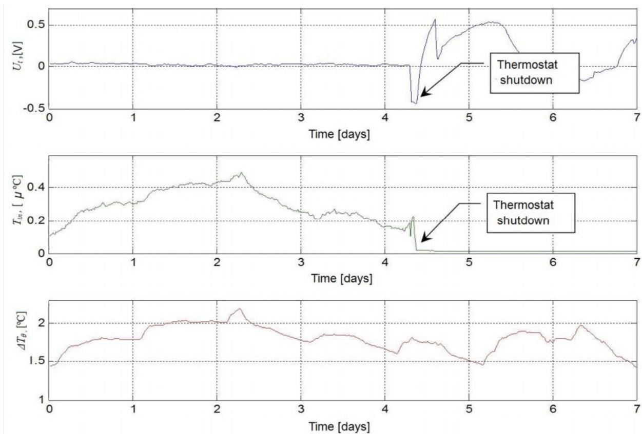
Fig.3. The suppression of thermal noise the KST-1 gyrotiltmeter with active thermostat [3]
