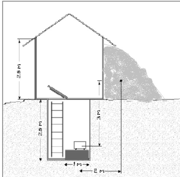
Fig.5. An example of the emergence of mass (snow drift) near the seismometer. The scheme of the station is taken from [6].
