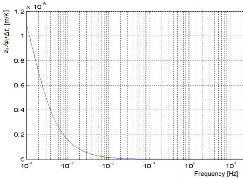
Fig. 2. An example of constructing of the noise transfer function generated by the temperature variation of the linear dimensions, in relation to the amplitude of ambient temperature changes (for the seismometer SK-1).
