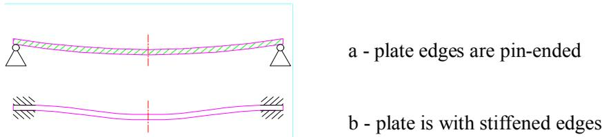
Fig. 4. Deformation of the device basis of various models.
