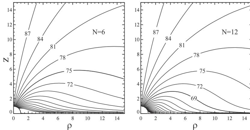
**Figure 2.** Contours of constant values of the function  $\Theta(r, \theta_0)$ , for different values of the foot point colatitude  $\theta_0$ . The two panels correspond to (left)  $n = 6$  and (right)  $n = 12$ ; the heavy lines on the plots show the shape of the surfaces, used for approximating the Region 1 and 2 field-aligned current sheets, respectively.
