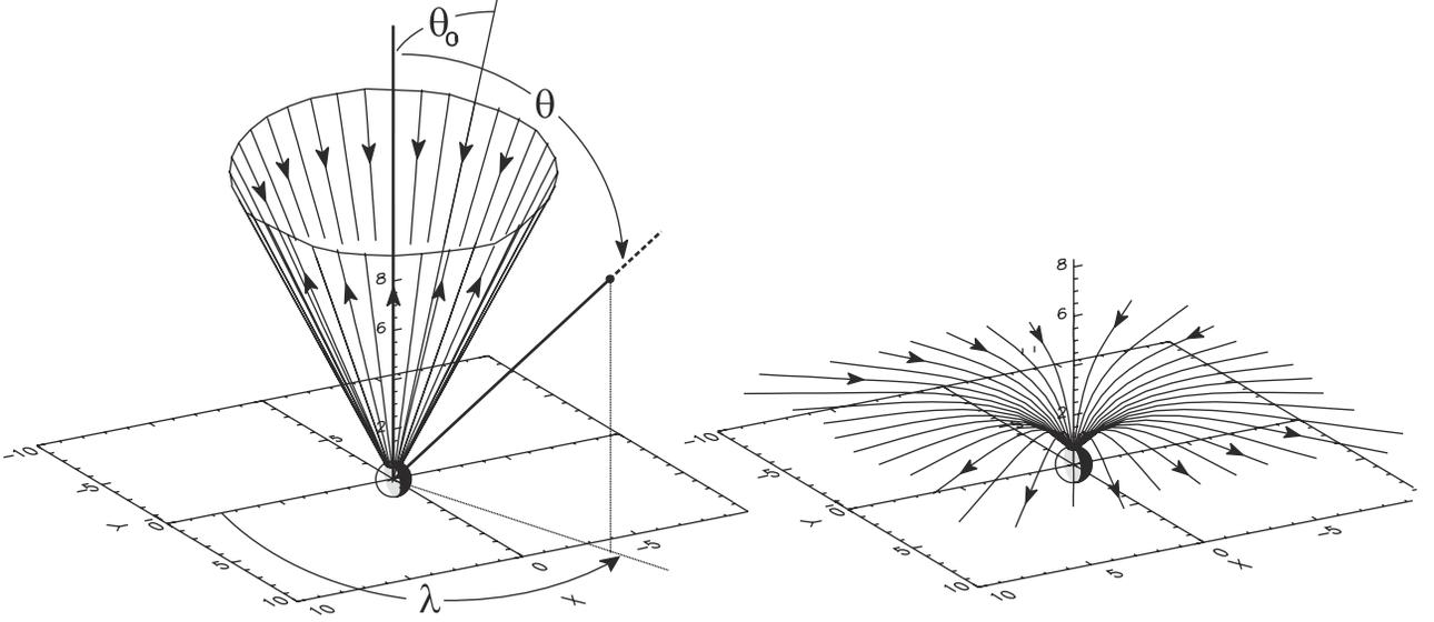
**Figure 3.** Illustration of the geometry of the model Birkeland currents: (left) a conical current sheet, whose magnetic field is given by the analytical vector potential (equations (16) and (17)) [Tsyganenko, 1991], and (right) a deformed conical sheet, in which the currents near Earth flow along dipolar magnetic field lines.
