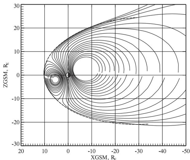
**Figure 9.** Field lines of the model ring current (axisymmetric part), shielded inside the model magnetopause. The ring current is coaxial with the Earth’s dipole, tilted in this example by  $\Psi = 20^\circ$ .
